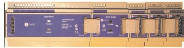
Power Supply Module System Module Feeder R1 Priority 2 Feeder R2 Priority 6 Feeder R3 Priority 14
